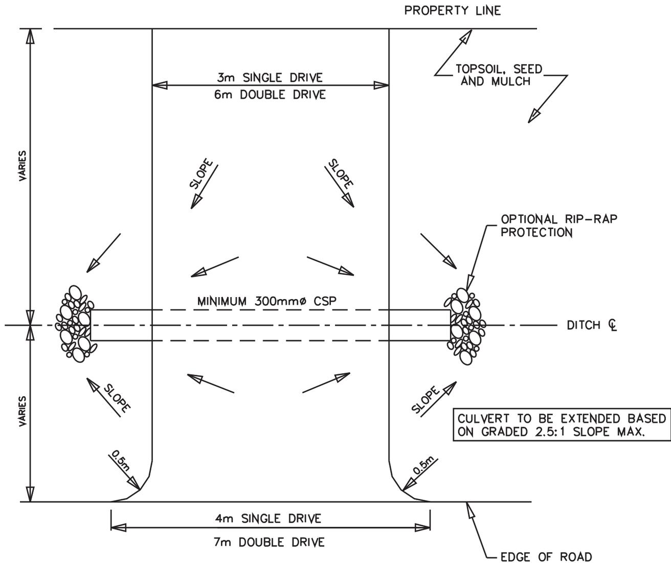
**NOTE:** CULVERT INVERTS, DITCH INVERTS AND SLOPE GRADES TO BE SHOWN ON APPLICATION DRAWING. ELEVATIONS TO BE RELATIVE TO CENTRELINE OF ROAD DATUM.
